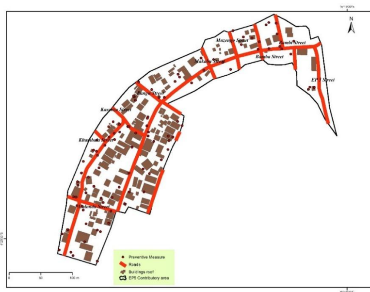
Fig.2b: Location of structures and measures for erosion control in the contributing areas of EP5 Livulu
